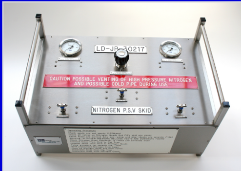
Pneumatic control panel for BHP Billiton Petroleum. Destined for three off shore rigs and were used for pig purging, 250 bar rated and regulated to 10 bar.
