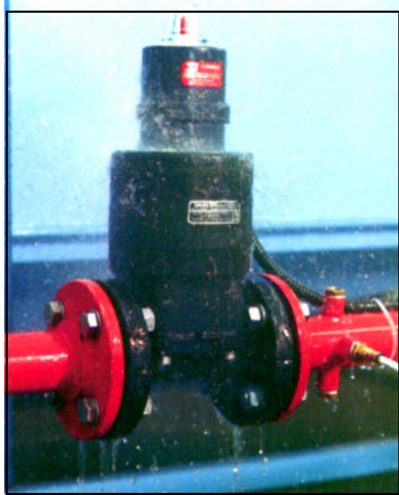
The EC 66 Switch Box undergoing weather proofing
